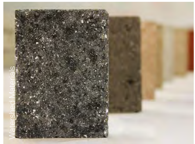
Figure 92: Example of rice husk ash bricks
