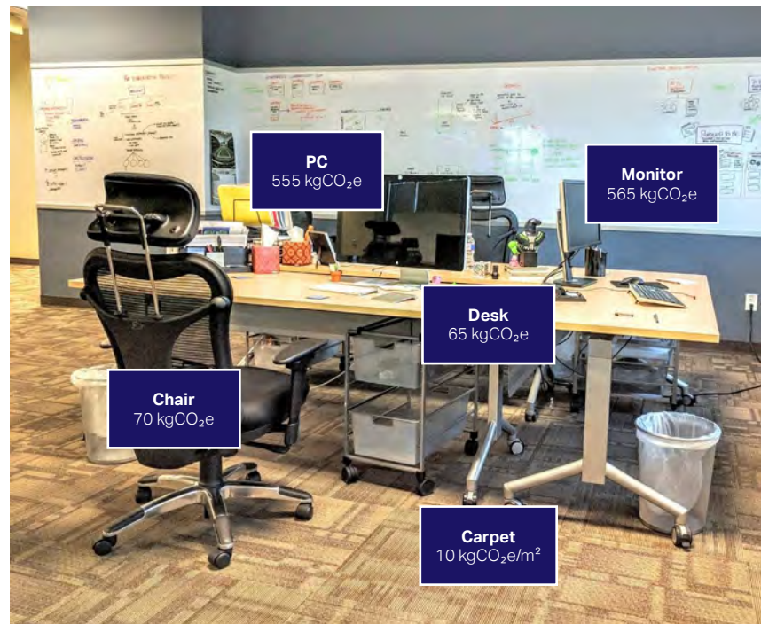
Workstation, 60-year lifecycle. PC, monitor, desk and chair replaced every 5 years. Carpet replaced every 10 years.
