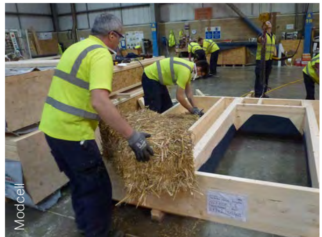
Figure 90: Example of straw bale modules
