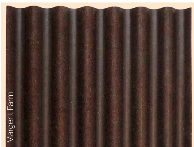
Figure 93: Example of hemp corrugated sheet
