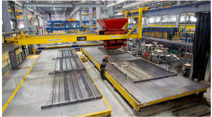
Figure 27: Laing O'Rourke Explore Plant robotically manufacturing precision reinforced concrete building units.
