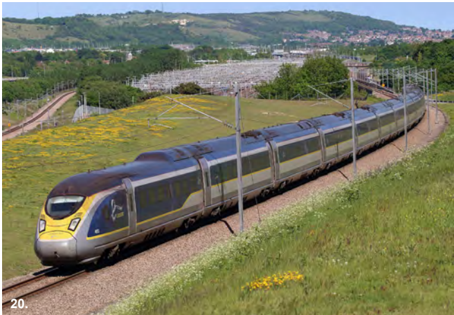
The new Velaro train is heavier than the model it will soon replace, which will affect track longevity
