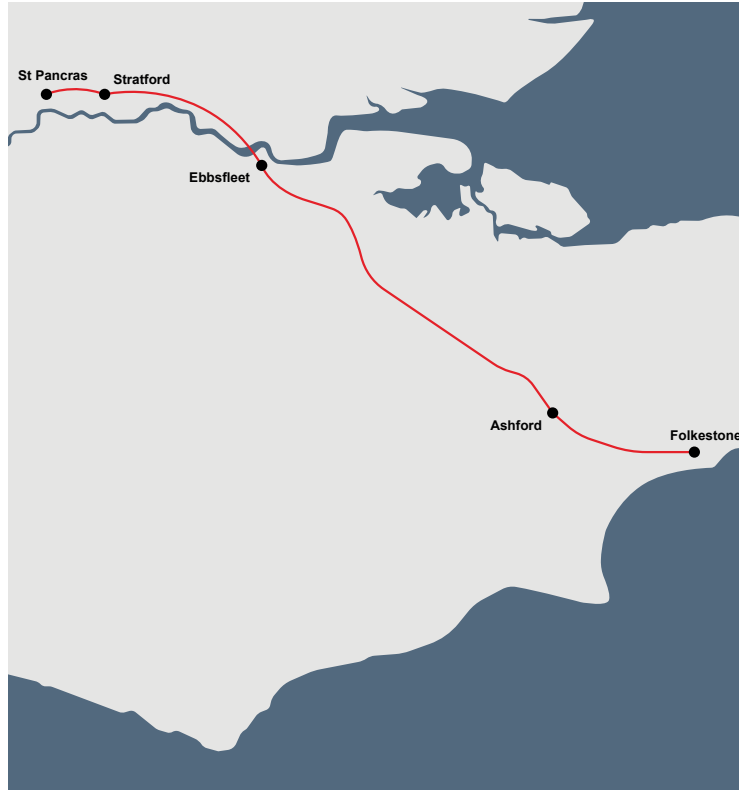
The 109km route of HS1 links the English end of the Channel Tunnel to central London
