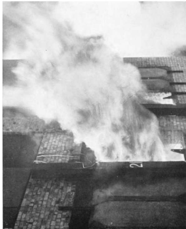
A. LOAD OF 1744 KG WITH 2.6 M 2 WINDOW AREA (TEST V)
