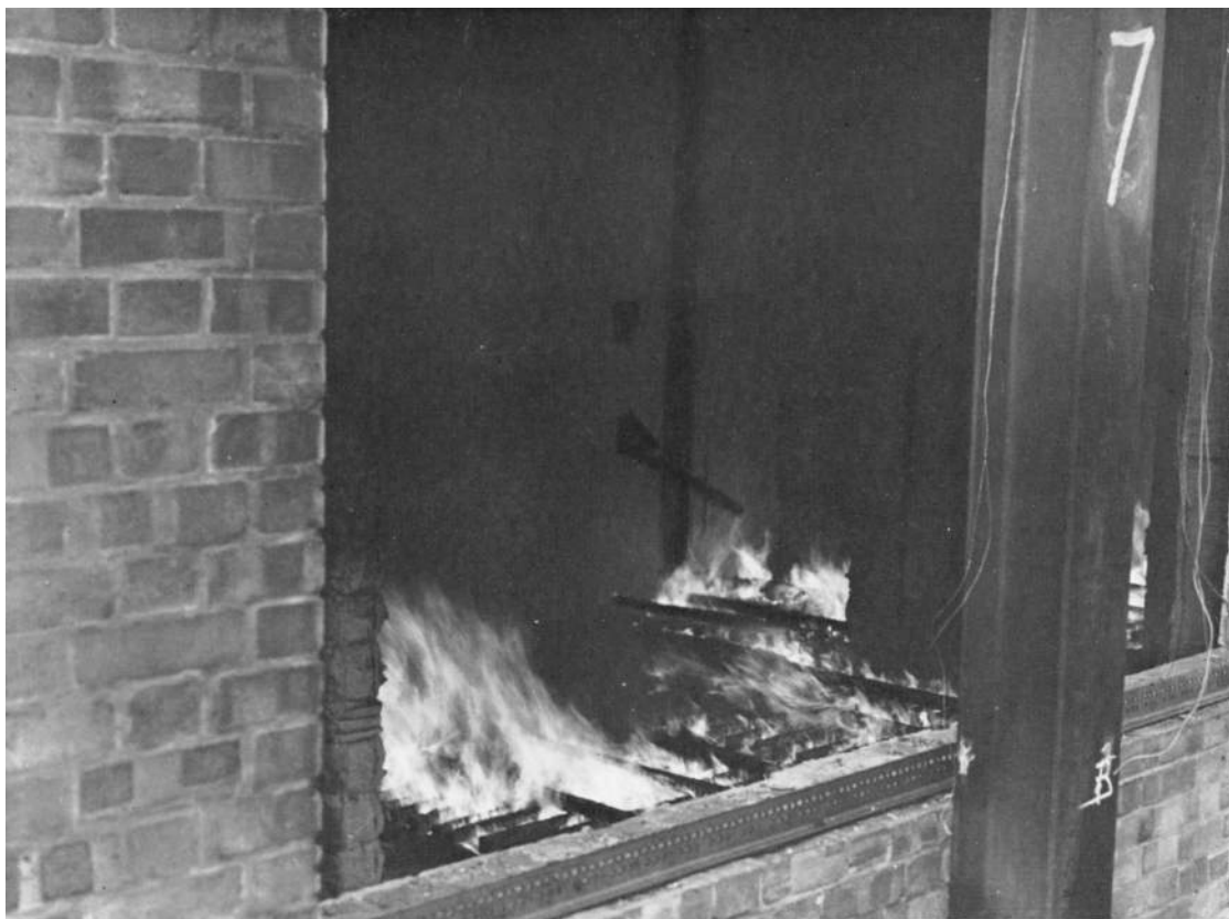
B. LOAD OF 218 KG WITH 11.2 m 2 WINDOW AREA (TEST K)
