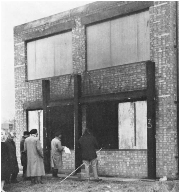
A. BUILDING USED FOR TESTS SHOWING THE SHUTTERS WHICH REDUCE THE WINDOW AREA TO 5.6 m 2
