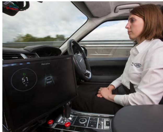
4: CAVs can show when emergency vehicles are approaching 5: Jaguar Land Rover's Advanced Highway Assist can autodrives, overtake and detect vehicles in the blind spot 6: Testing at the HORIBA MIRA facility demonstrated a system that notified drivers of nearby emergency vehicles 7: The emergency brake warning system in use
