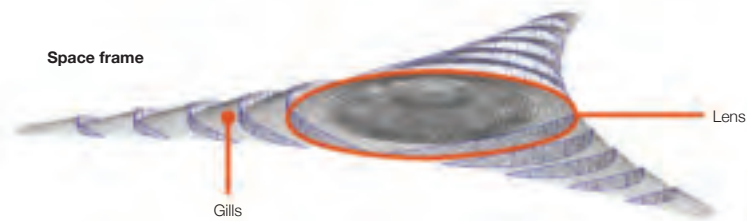
Gill columns and perimeter beam
