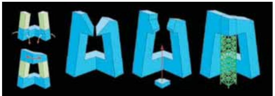
5. Three alternative methods of constructing the Overhang.
