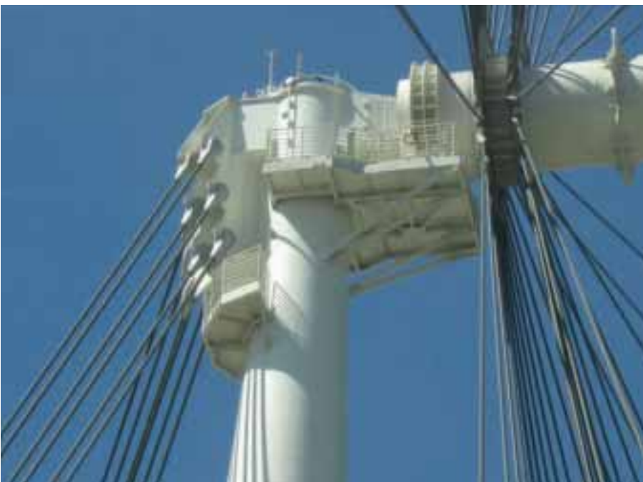
18. The main spindle is 2.6m in diameter, 25.25m long, and weighs 180 tonnes.
