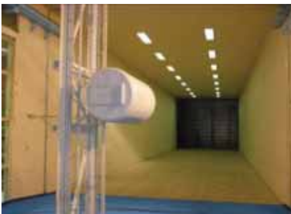
22. Capsule and rim segment during wind tunnel testing.
