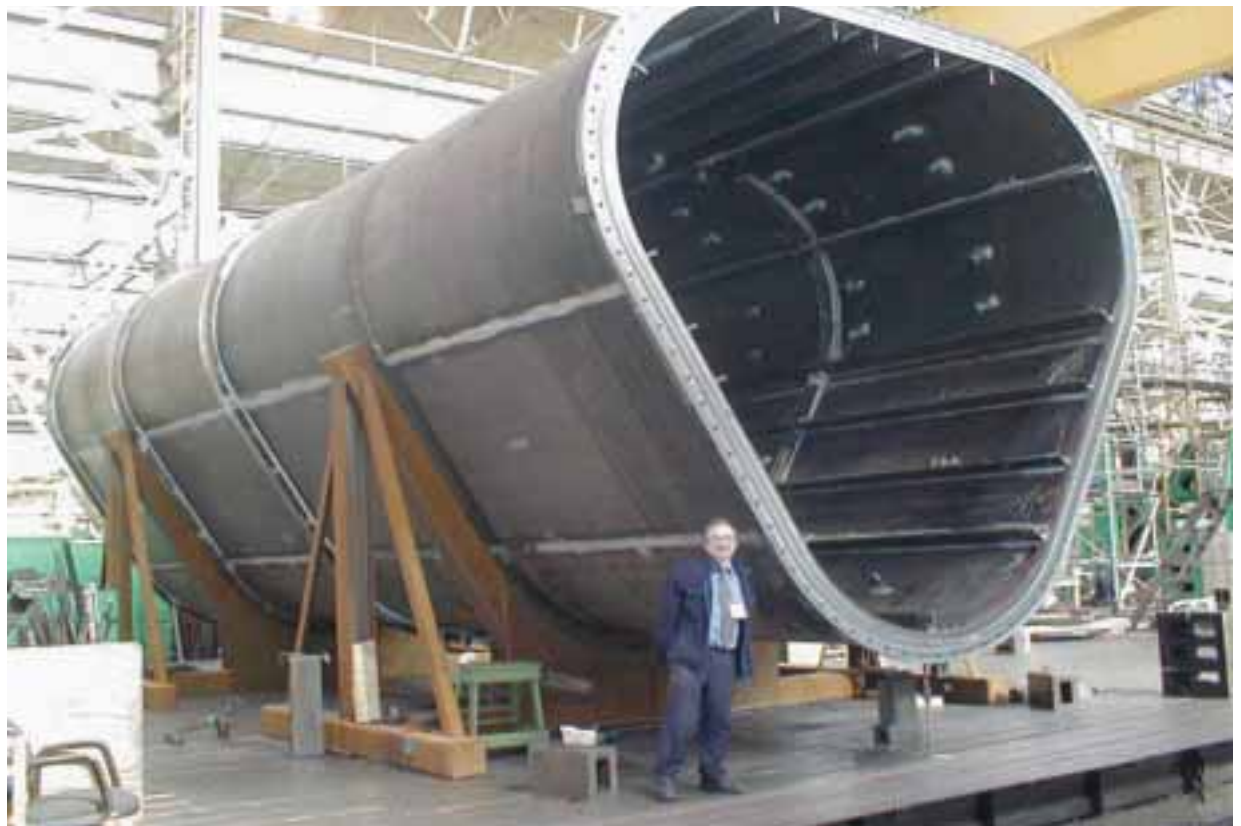
8. Prefabricated mast section before installation of stairs and lift risers.
