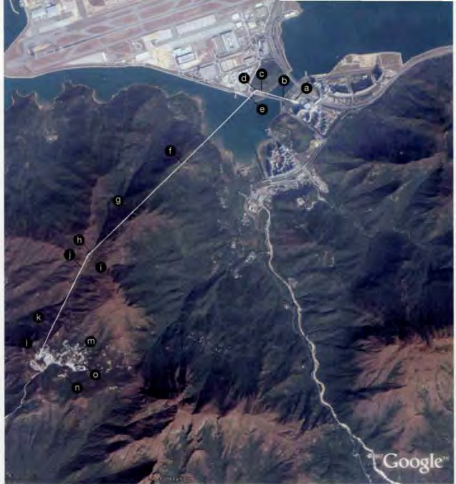
4. Route alignment for the cable car system: (a) Tung Chung terminal, (b) Tower 1, (c) Tower 2A, (d) Airport Island angle station, (e) Tower 2B, (f) Tower 3, (g) Tower 4, (h) Tower 5, (i) Nei Lak Shan angle station, (j) Tower 6, (k) Tower 7, (l) Ngong Ping terminal, (m) Ngong Ping Village, (n) Tian Tan Buddha, (o) Po Lin monastery.
