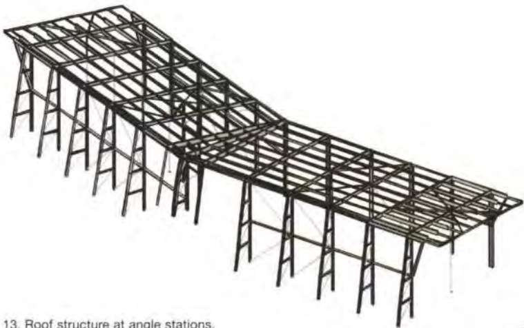
13. Roof structure at angle stations.
