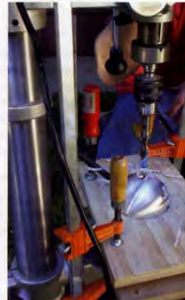
4. Drilling an aluminium node.
