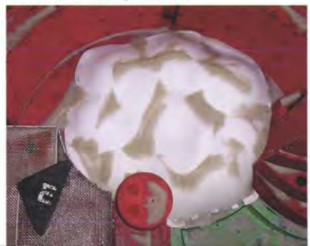
29. Snow drift modelling in water flume.
