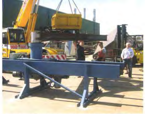
11. Prototype load-testing of Traveller bogies at the Danfab workshop. (Garry Ormsten, project architect, in background).
