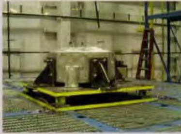
21. Ball-in-box dampers were mechanically and acoustically tested at the State University of New York at Buffalo to verify their engineering design properties.
