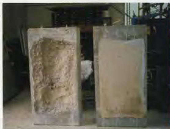
14, left: Concrete samples after exposure to a 1200°C fire for two hours. The plain sample (left) suffered from explosive spalling and severe section loss, while the one with polypropylene fibres (right) had only minor surface cracking.
