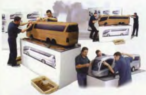
5. Developing the 1/6 scale models of the coach.
