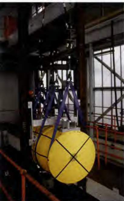
8. Drop test of a 500 litre drum.
