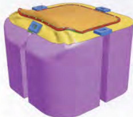
9. Finite element impact analysis of the Nirex 3m 3 box - at the end of a 25m drop.
