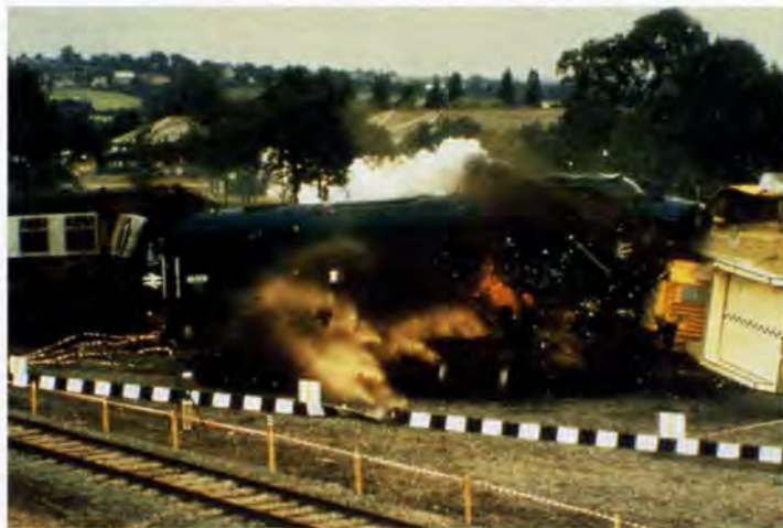
1. Train crash demonstration of the Magnox flask.
