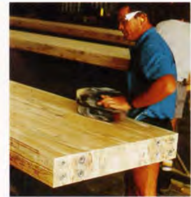
11. Threaded couplers recessed into ends of glulam member.
