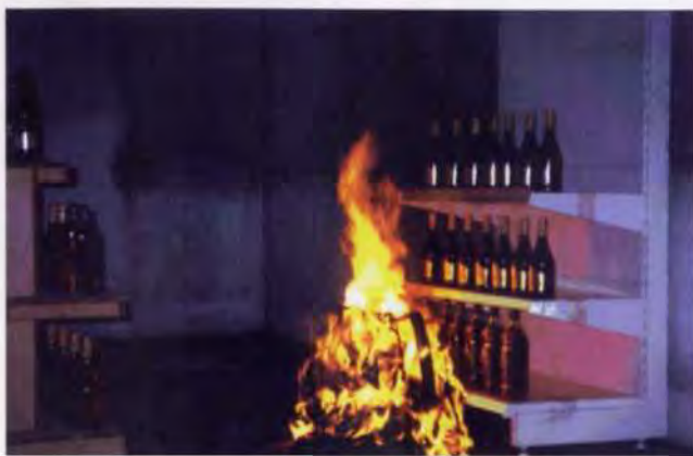
4 left: Test fire in mock-up of duty-free area.
