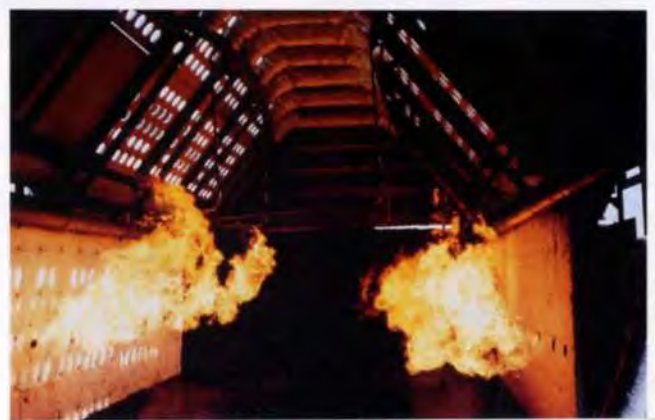
4 left: Test fire in mock-up of duty-free area.
