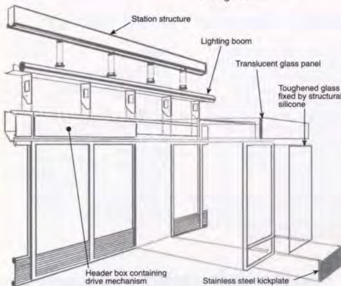
1. Exploded view of door system.
