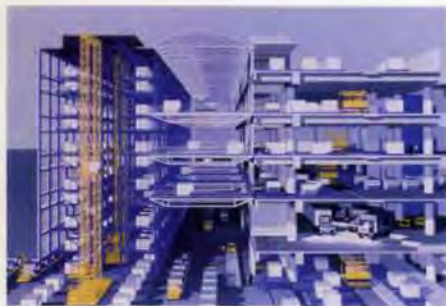
5. Computer-generated image of part of the Terminal, showing (l-r) stand-alone container storage (CSS), 'roadway', operations and truck dock levels.
