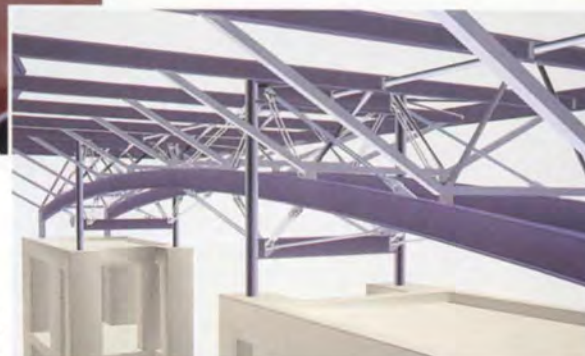
7. 3D computer-generated image of external lobby truss.
