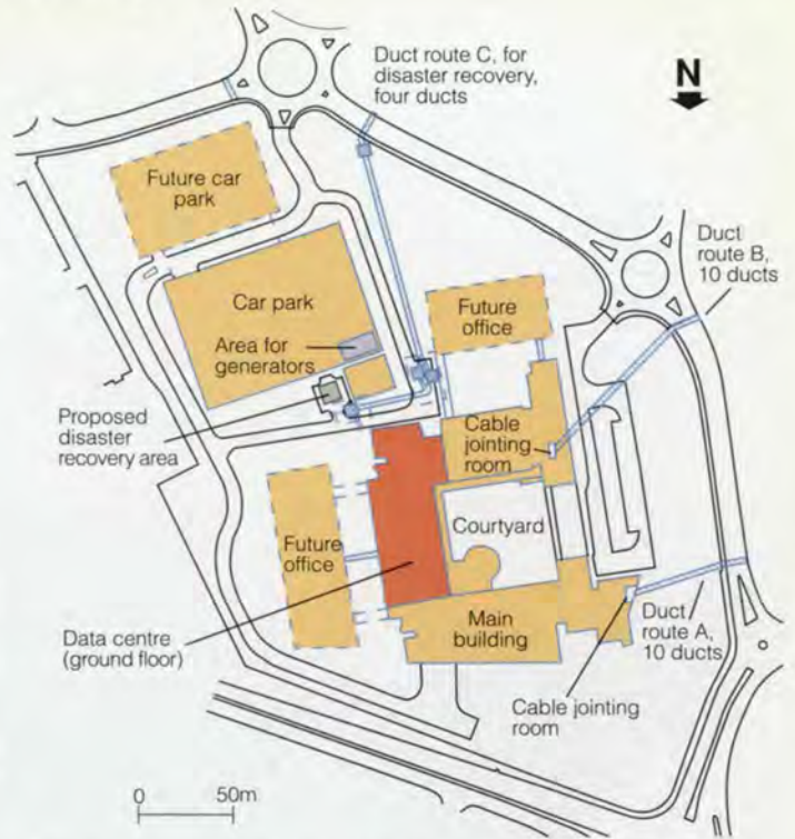
2. Site plan, showing ducts and cable entry.
