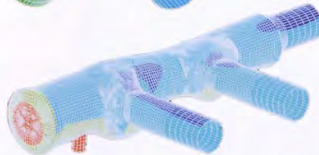
5 & 6. Left and below: Finite element meshes for Terminal 4 and Terminal 1 chambers. (not to the same scale).
