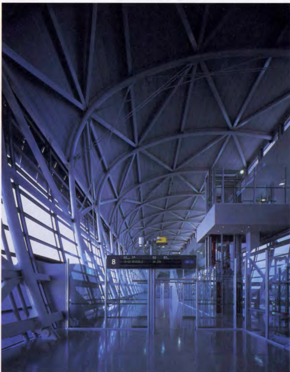
13. 'Fish tail' ducts supply air to Wing.
