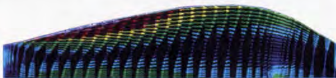
A. CFD air movement analysis assisted in choice of roof geometry.
