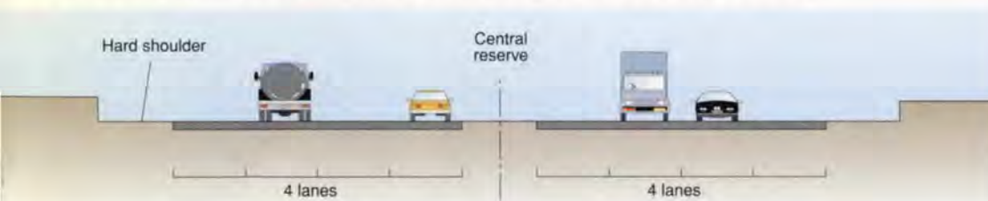
3. Above: existing dual three-lane motorway; below: symmetrical widening without land take (rapid widening).
