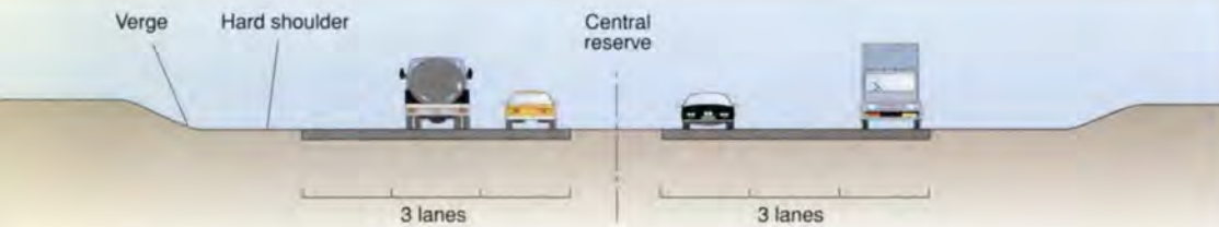
3. Above: existing dual three-lane motorway; below: symmetrical widening without land take (rapid widening).
