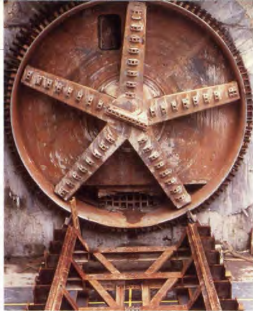
2. Tunnel boring machine.
