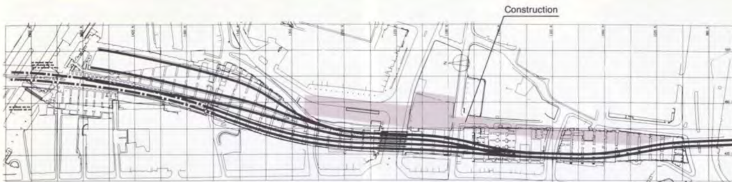
16. Temporary track alignment: Stage 1.
