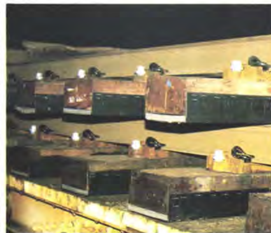
8. Under-sleeper isolators stacked (Photo: Ove Arup & Partners).
