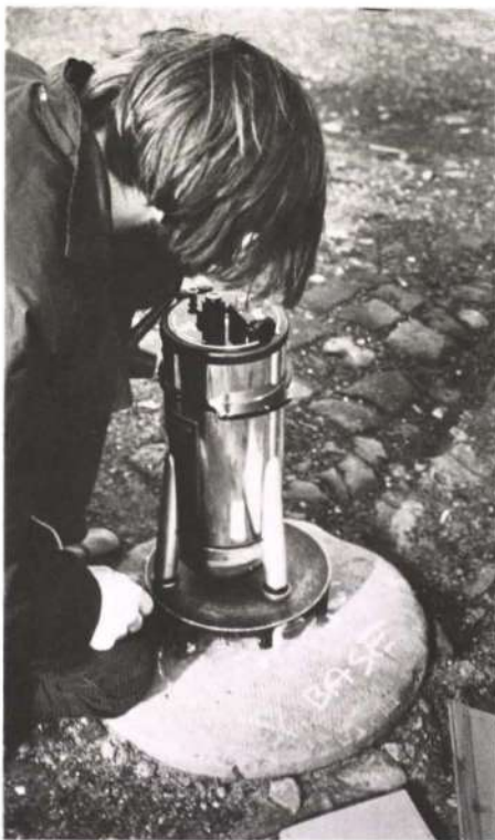
Fig. 2 The gravity meter, levelled upon its tripod, being read at this site's base station (Photo: Carl Poster)
