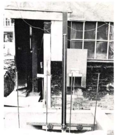
Fig. 18 Water level tube and control box for pier 8, and levelling tape. (Photo: Stan Parkinson)
