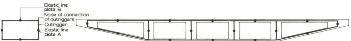
Cross section of space frame representing single cell box.
